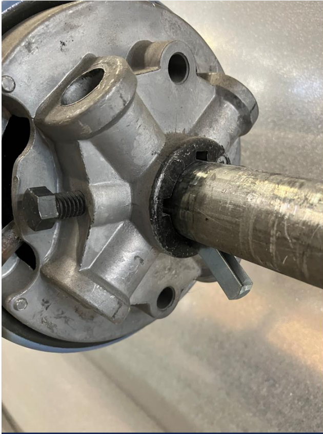
11. Stretched spring: with wedge and 2 set crews.
