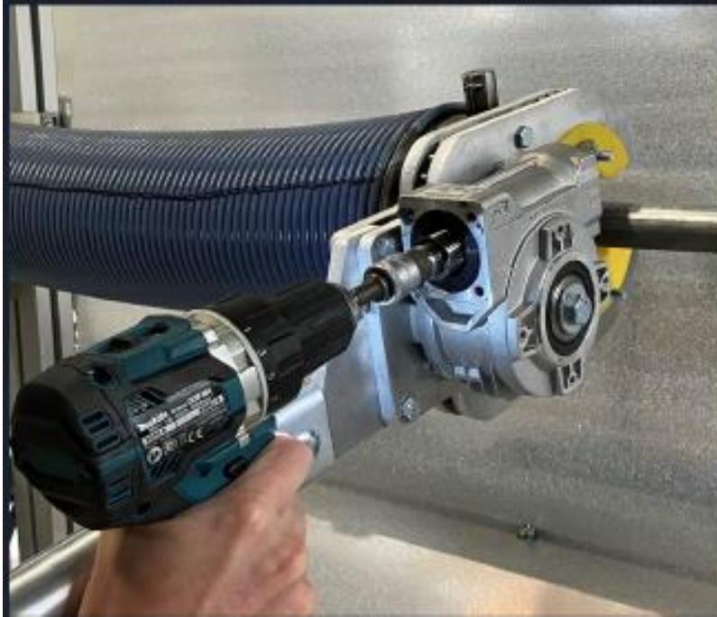
Figure 2 Application of the Industrial torQtool 2 using a drill: the spring is tensioned by the drill bit drive and not by manual force.
